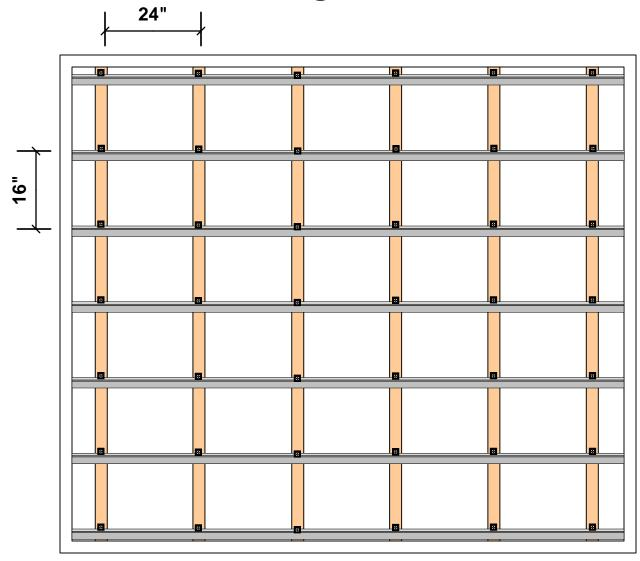
APPLICATION RECOMMENDATIONS FOR CEILING, WOOD OR STEEL FRAMING.
