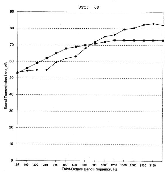
→ Sound Transmission Loss (dB) - Limiting STC Contour
