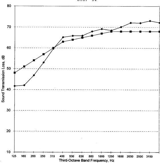
→ Sound Transmission Loss (dB) - Limiting STC Contour
