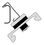
Rotate clip under CRC channel
