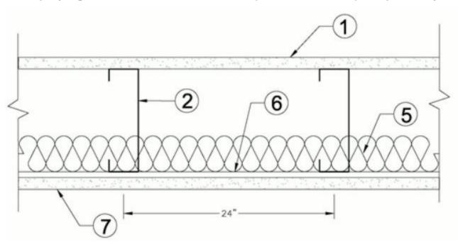
1. **Flooring System - Building Units\*** — Nom 3/4 in. thick, tongue and grooved boards. Long dimension of boards to be perpendicular to joists with end joints staggered a min of 4 ft. and centered over the joists. Boards secured to steel joists with 1-1/4 in. long self-drilling, self-countersinking, bugle head steel screws spaced a max of 12 in. OC in the field with screws located 1 in. from long edge, and max 8 in. OC along the end joints with screws located 1/2 in. from end joint.
